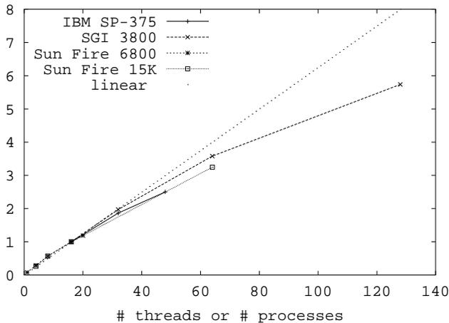
Fig. 8. Speedup of SPECcenv for the medium data set normalized by the 16-way speedup.
