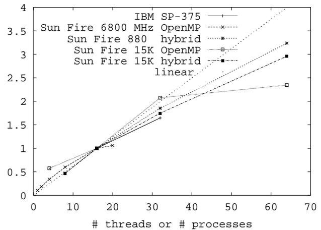
Fig. 10. Speedup of SPECchem for the medium data set normalized by the 16-way speedup.
